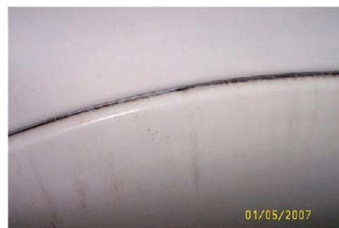
Figure 4. Staining of vessel’s walls post Buchwald–Hartwig reaction and scavenging.
